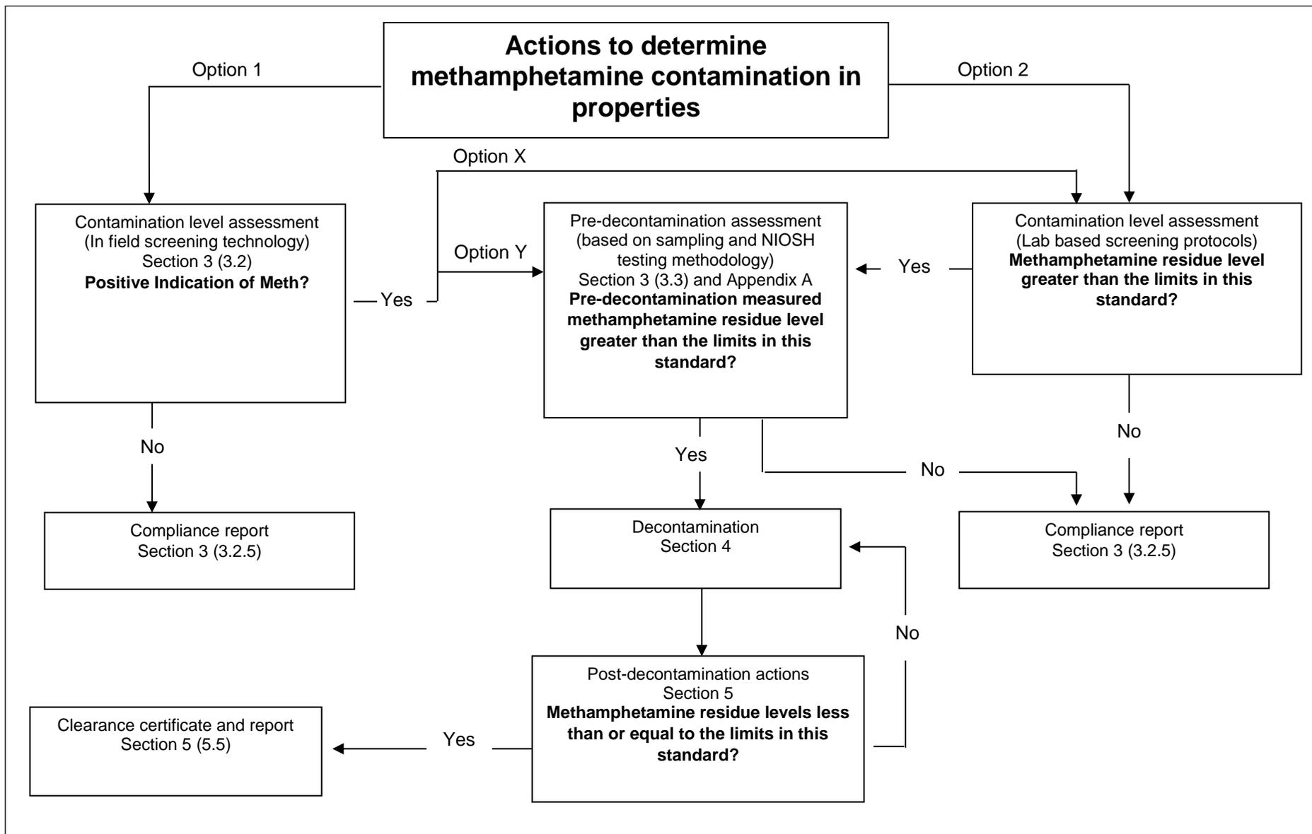
Figure 2 – Actions to determine methamphetamine contamination in properties
